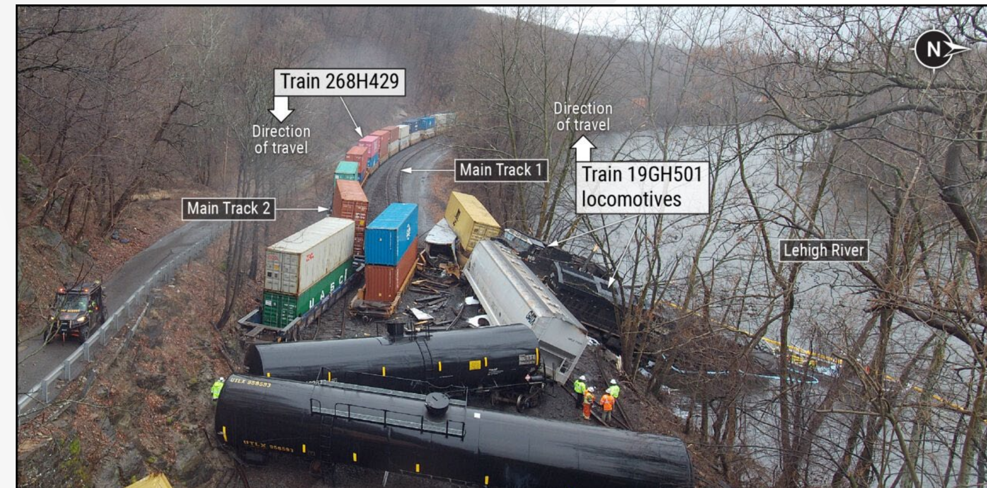
A train derailed and another struck the railcars in Easton, Pennsylvania near the Allentown Road Subdivision on March 2, 2024. The two derailed locomotives partially submerged in the Lehigh River and discharged locomotive diesel fuel into the water way. (Photo courtesy of Lehigh County Emergency Management, NTSB )
